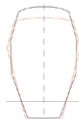
Hull Cross Section Comparison with Janus (in red)
