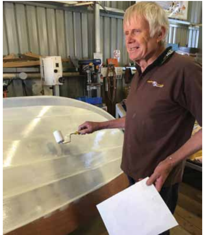
Note David's smile of 'OH NO!' revelation! Palette MUST be held more or less level, or else you will get paint, as David Hinves found out, in your sock! First coat, note shadows. Subsequent thin coats fix that quickly.
