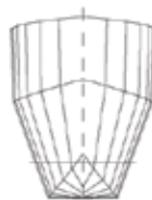
Hull Cross Sections (aft on left, fwd on right)
